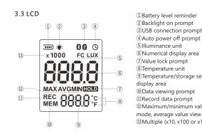
4 Auto power off prompt ⑤Illuminance unit 6 Numerical display area 7 Value lock prompt ®Temperature unit Temperature/storage serial number display area
